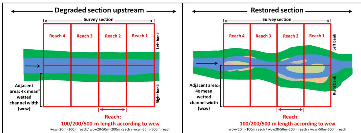
**Figure 2-1: Delineation of survey sections and reaches for the field assessment in the degraded (left) and restored (right) sections.**
