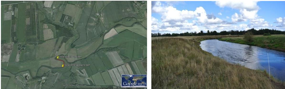
**Figure 12-14 Small restoration project DK\_R2. Overview of the site restored in River Storå (left) and closer view on the gravel bar created in 2011 by addition of coarse material (right) (Niels Bering Ovesen)**
