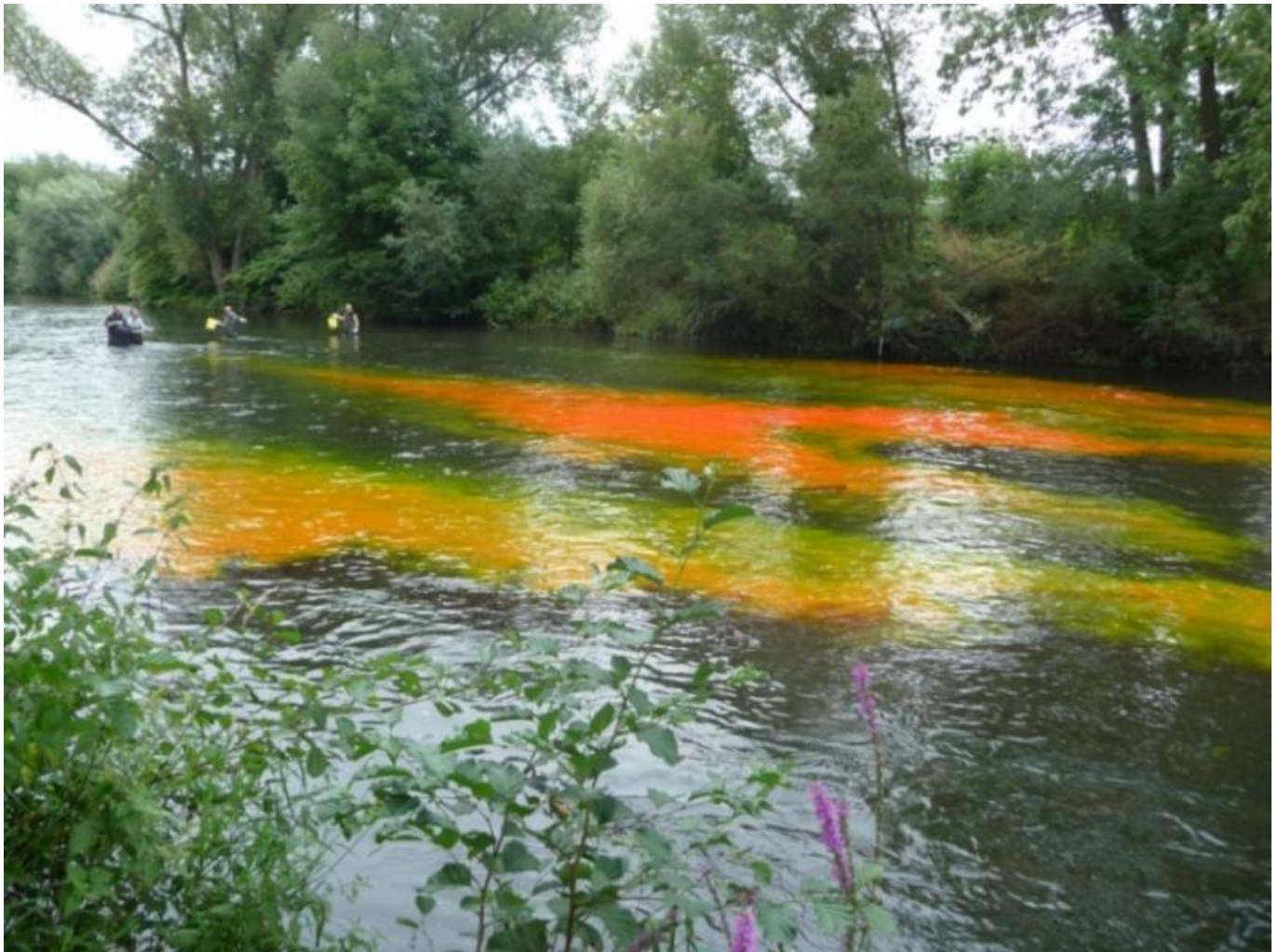
Figure 2: Injection of a conservative tracer (Amidorhodamin G) (photo: Benjamin Kupilas).
