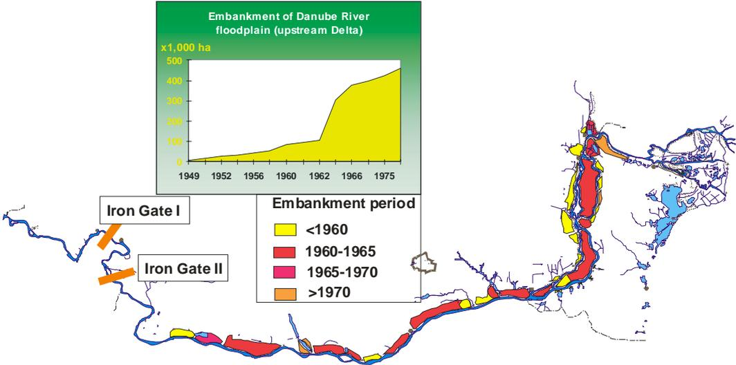
Figure 7.4 The main hydromorphological changes in the Lower Danube, upstream Danube Delta: floodplain embankments and impoundments at Iron Gate I and II (Schiemer et al. 2004).
