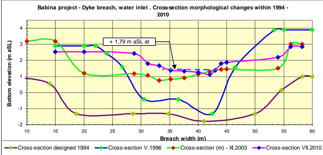
Figure 7.14 Sedimentation process at the water inlet cross-sections, Babina project
