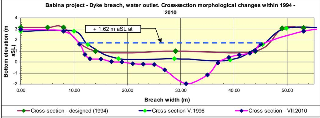
Figure 7.15 Sedimentation process at the water outlet cross-sections, Babina project
