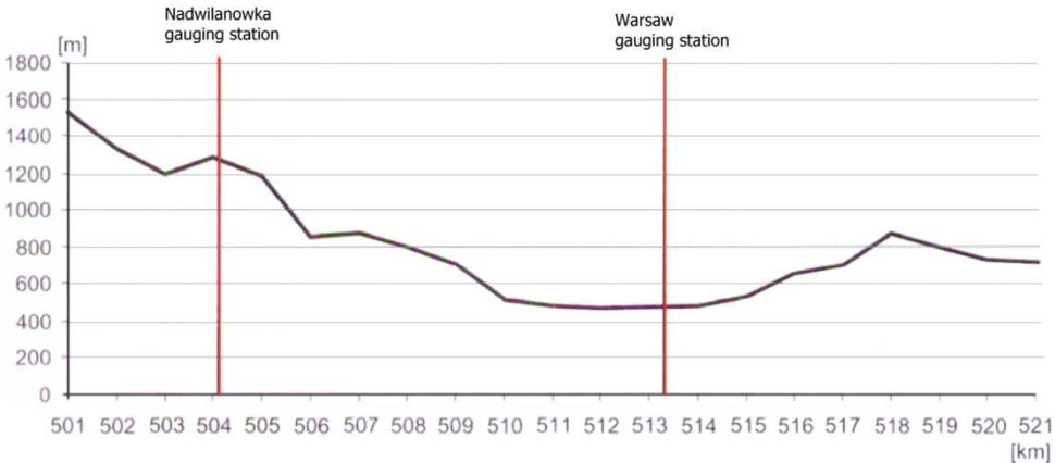
Figure 6.11. The flood channel width limited by embankment on the Vistula River reach near Warsaw (Magnuszewski 2013)
