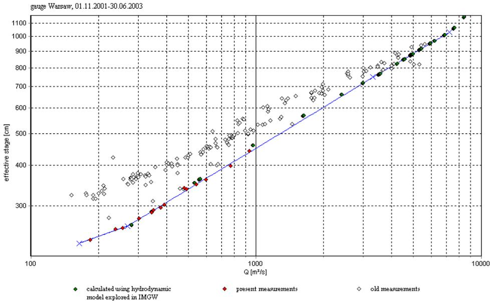
Figure 6.21. Stage - discharge curve for the Warsaw gauge station, located in km 513 (Zelazinski et al. 2005)
