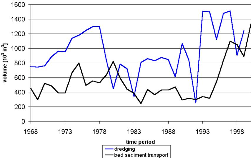
Figure 6.23. Comparison of dredged sand volume with the volume of computed bed-material sediment transport in the Vistula River in period 1968-2000 (Zelazinski et al. 2005)
