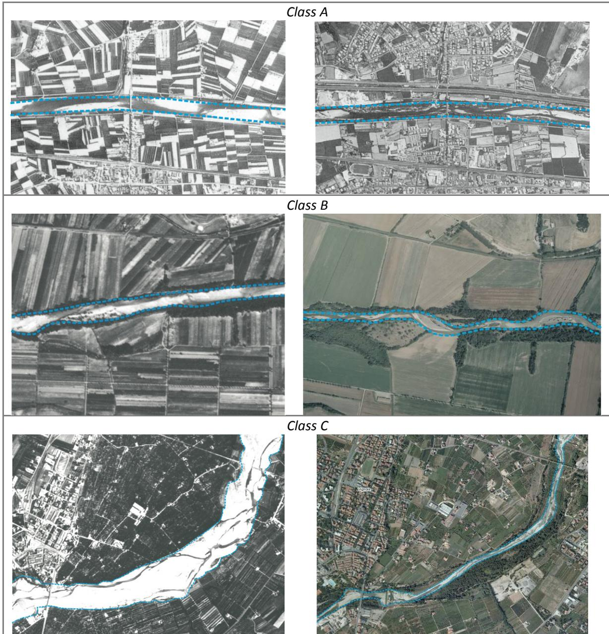
**Figure A3.64 Adjustments in channel width.**
